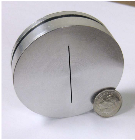
Fig. 5 Actuator with a rectangular slot orifice along side a dime provided for scale
